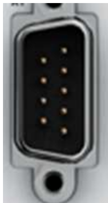
Figure 3 CANopen connector plug
