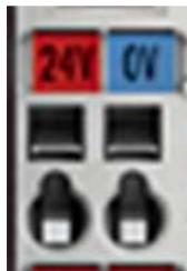
Figure 2 Power input terminals
